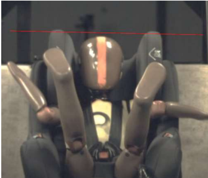
Figure 5: Perimeter surrounding the dummy's head in a forward-facing CRS at the completion of the post-impact phase
